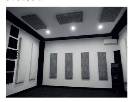
**Studio B** is 6.6 x 6.6 meters with ceiling height of 4 meters. It's a room within a room design with extensive acoustic treatment, created one piece at a time and tested to ensure the acoustic performance was complementary. Addition 8 xlr microphone lines + 4 instrument sends piggy backing to and from Studio A. Studio B makes the perfect DIY workshop recording room or rehearsal space for bands on a budget.
